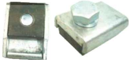
CR 80 Single Bolt Rail Clamp (M 20 Bolt) (Square Block 20 MM Thickness) Drg. No. AI/D/25 (B)
