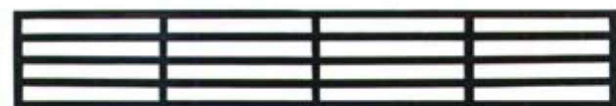
Walkway Jalli (Manufactured using MS square pipes)
