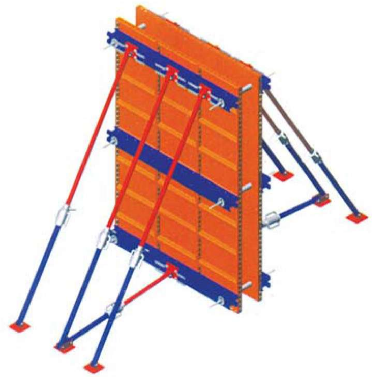
Wall formwork supported by Prop Struts
